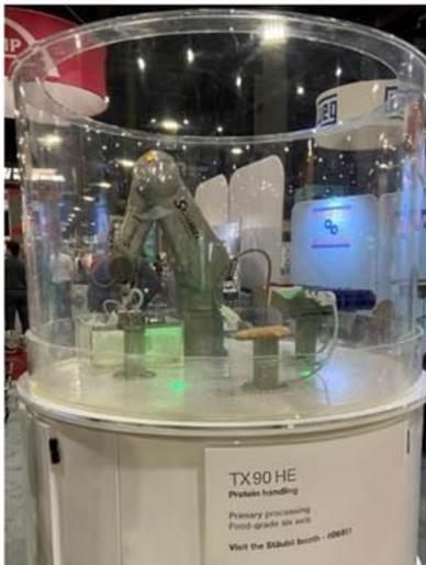
The Stäubli TX2 90 HE 6-axis robot demonstrates wash-down operations and waterjet cutting with two different protein products.
